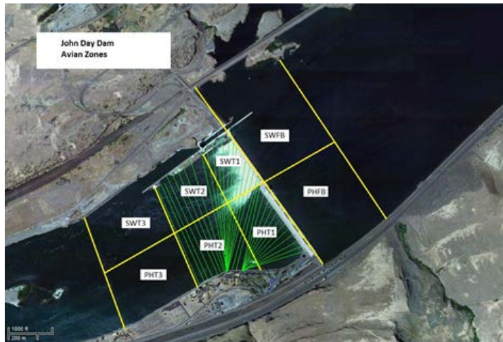
Figure 3: Avian array at JDA Tailrace BRZ installed in 2010 (Powerhouse Forebay-PHFB, Spillway Forebay-SWFB, Spillway Tailrace zones 1-3 [SWT1-SWT3], Powerhouse Tailrace zones 1-3 [PHT1-PHT3]).
